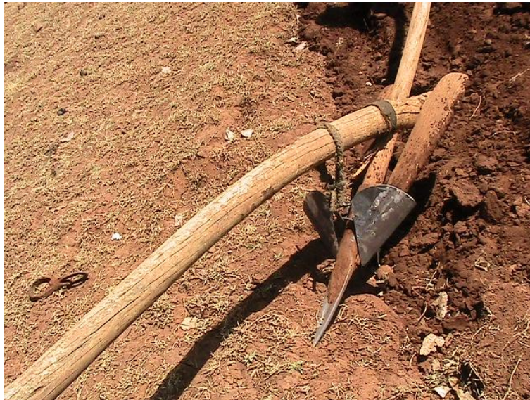
Figure 9. The Arashogel designed to avoid the traditional cross-ploughing during consecutive tillage operations due to its wings, which cut the grasses and other weeds left by Maresha. Unlike the traditional Maresha, this tillage implement enables to farmers to effectively plough parallel to bunds and terraces.
